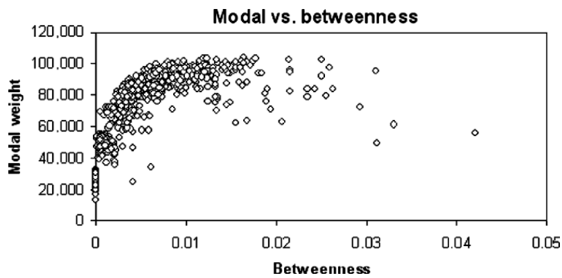
Fig. 5. Correlation between the modal weight and betweenness of the nodes in an ER graph (1000 nodes, average degree 3.5).
